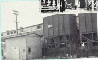
At the extreme left is the sand scrubber, then the cyclone and at the right our No. 7 Model 112 KD Dustube.
